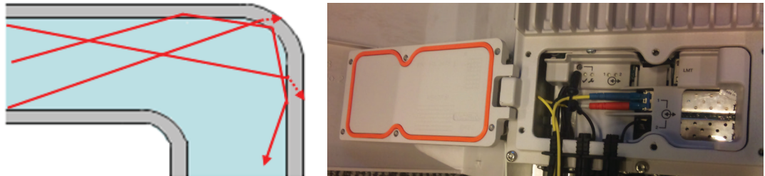
Figure 11. Macrobends typically found in RRU enclosures, junction boxes, and fiber trays
