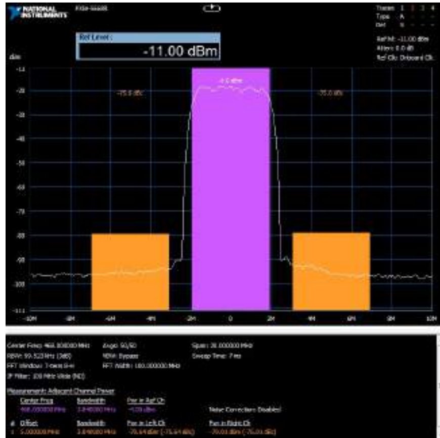
Figure 16: PXIe-5668R Measuring WCDMA ACPR with 100 MHz Wide IF Filter and Noise Correction Disabled
