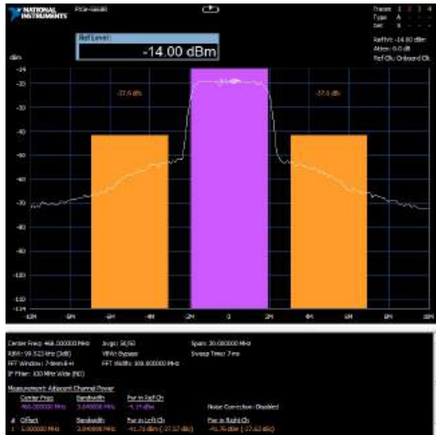
Figure 17: PXIe-5668R Measuring WCDMA ACPR showing ADC Distortion
