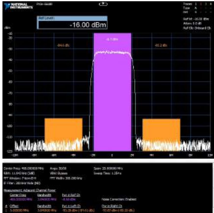
Figure 19: PXIe-5668R Measuring WCDMA ACPR with 300 kHz Wide IF Filter and Noise Correction Enabled
